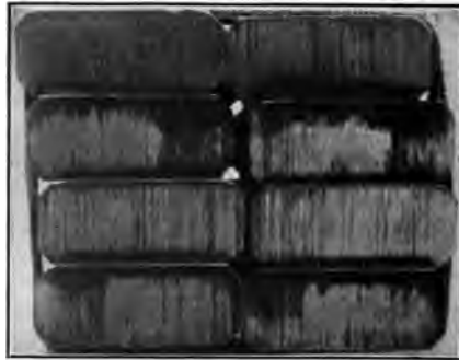
FIG. 97.—Coated brush surface caused by collection of dirt on commutator.
